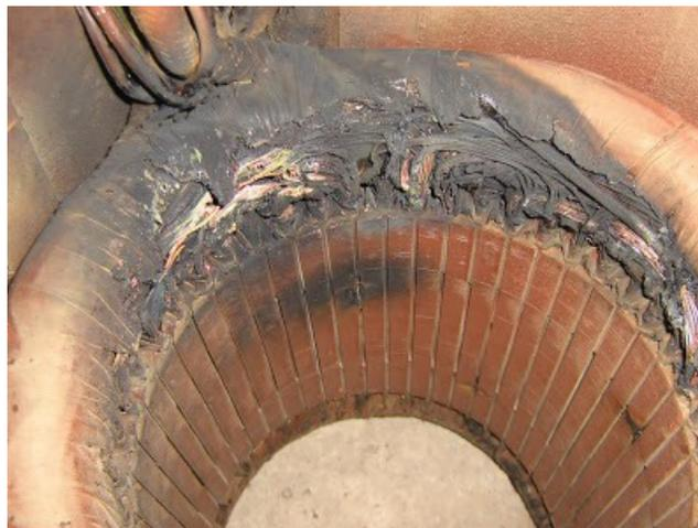
Figure 1. Defective Stator Winding of a Welding Alternator (Image Source: [WindingPhotos](#))
